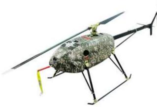
Max speed: **120 km/h** Practical ceiling: **5000 m** Flight time (max with 4 kg): **5h**
