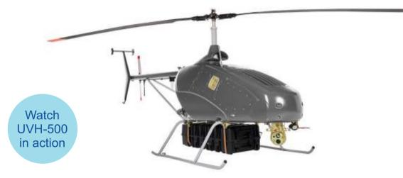
Endurance: 7 hours Operation Range : 850 km Max speed: 160 km/h Practical ceiling : 4500 m Temperature range : -35 °C...+50 °C Length: **7050 mm** Main rotor diameter: **6280 mm** Height: **2350 mm** Empty weight: **340 kg**
