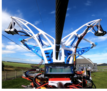
Fig. 5: Gripper engaged by powerline.
